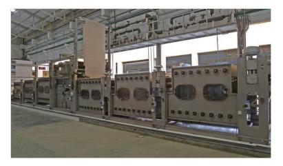
**Continuous processing** uses a series of vessels, each of which represents one processing step. Fabric is passed from one vessel to the next in the correct sequence for the processes being carried out.
