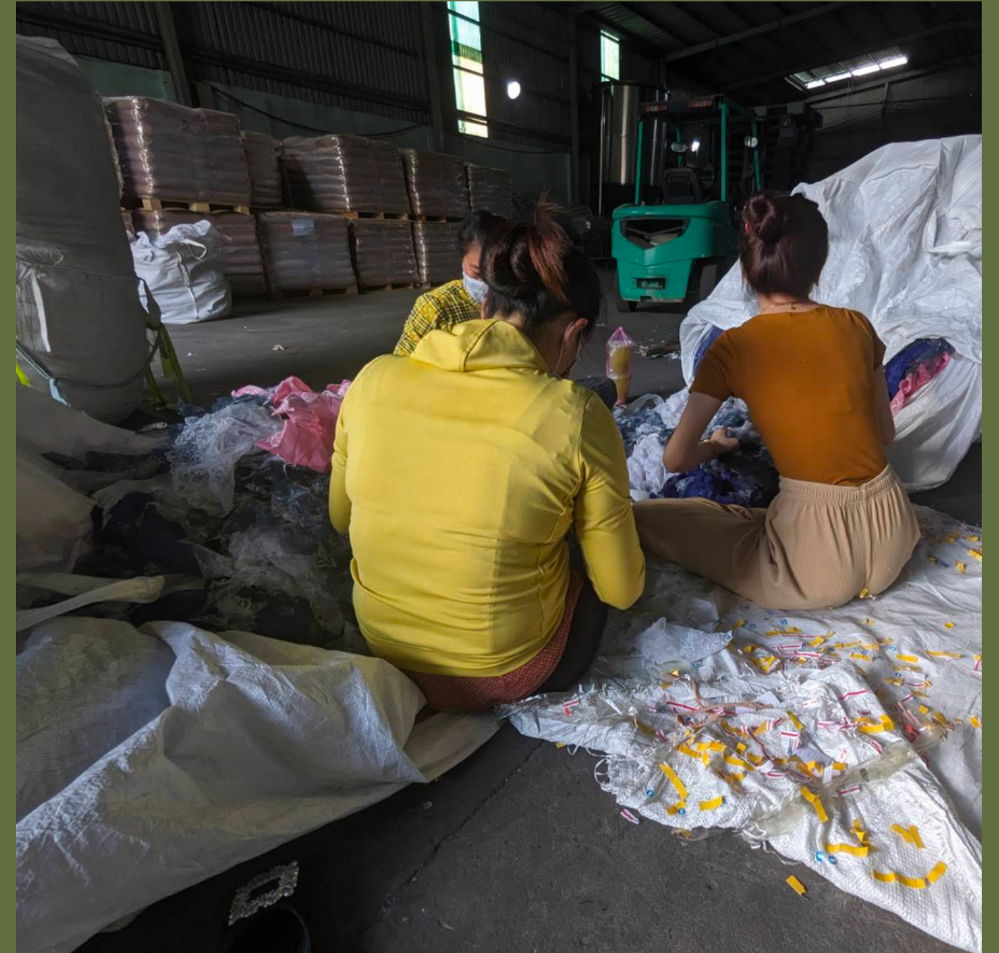
Scrap separation by fiber content
