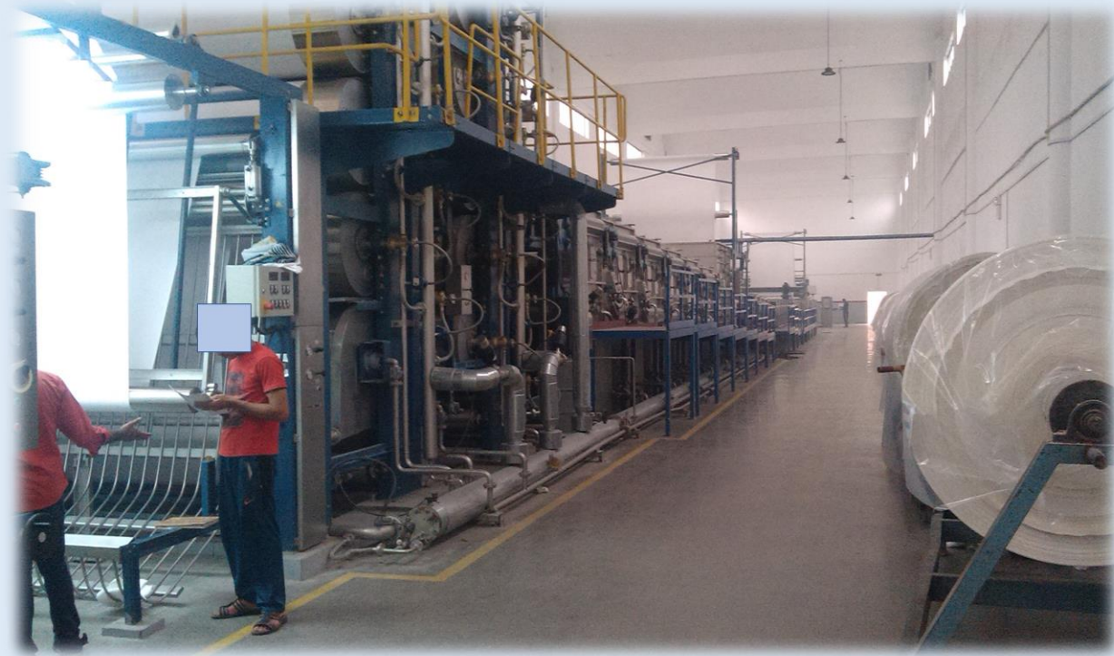
Figure-11: Example for mercerization machine for cotton woven fabric
