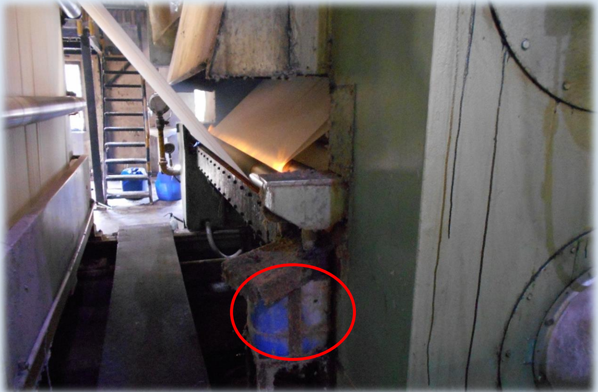
Figure-3: Singeing machine in operation with cooling water being collected in blue container and reused as showering water at singeing wet scrubber
