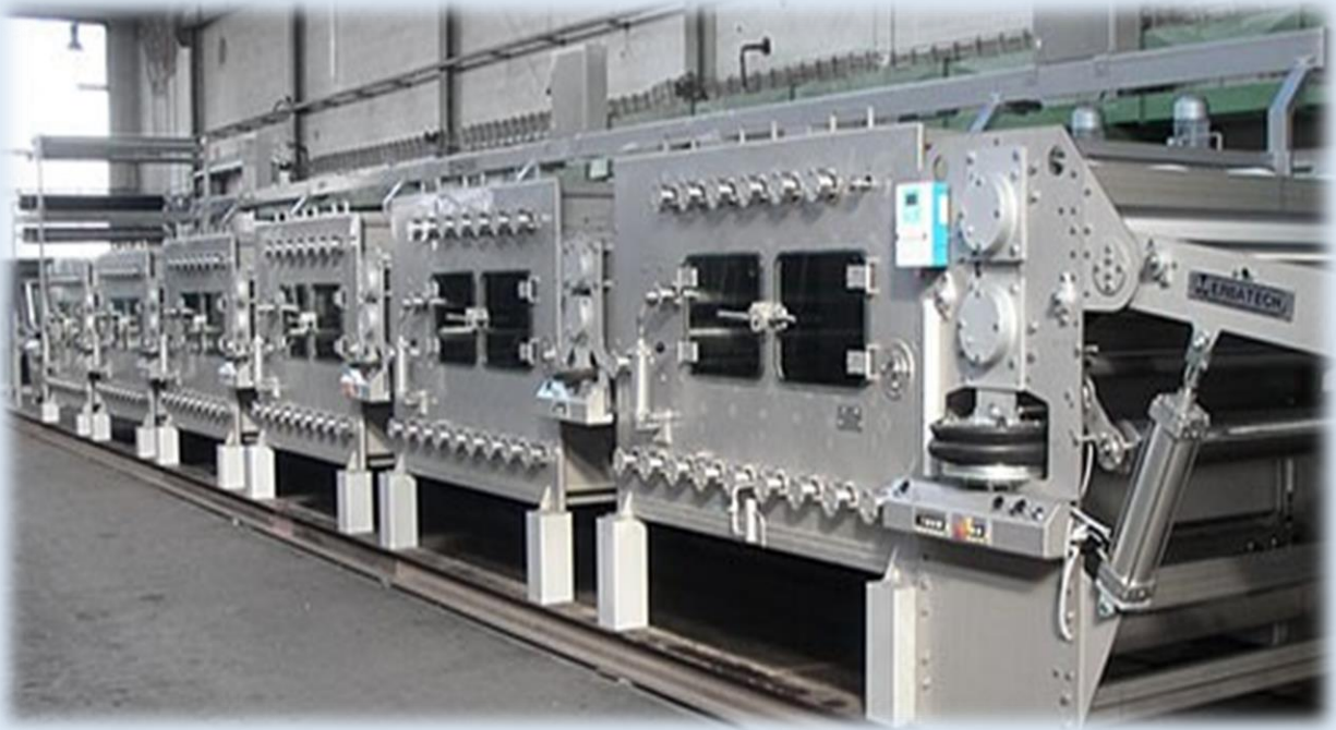
Figure-19: Wash boxes of continuous pre-treatment machine for woven fabric in counter-current washing mode
