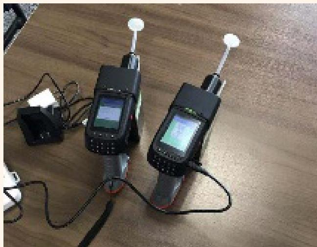
In order to conduct the VOC screening, you will need a PID-screening device (photoionization detection, please see photo).
