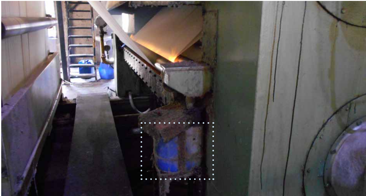
Figure-3: Singeing machine in operation with cooling water being collected in blue container and reused as showering water at singeing wet scrubber
