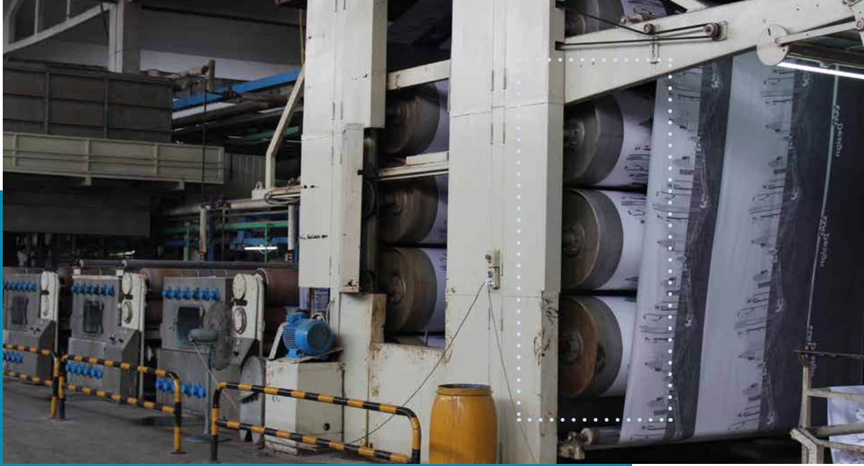
Figure-5: Cooling drums attached with pad steam dyeing machine
