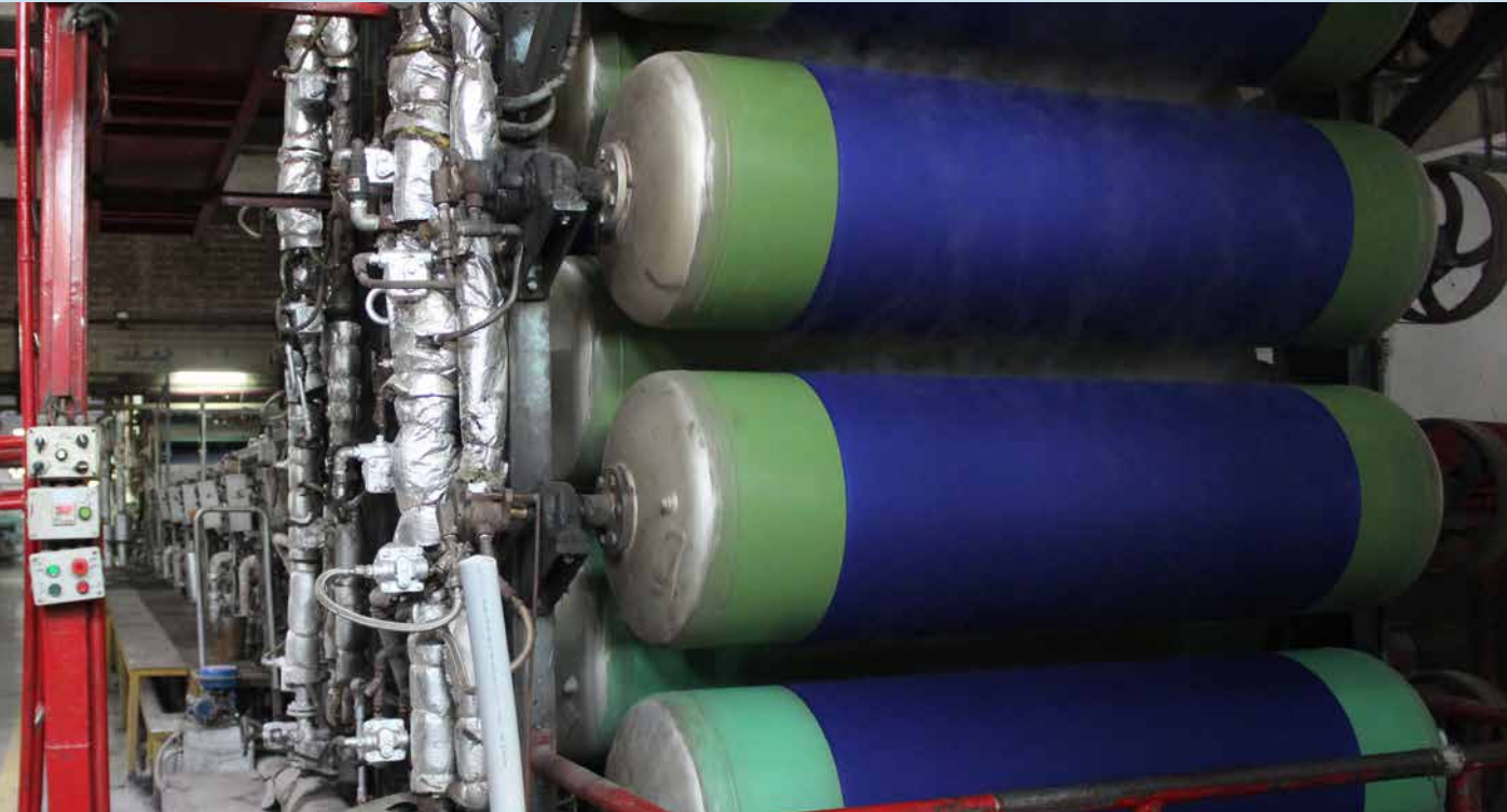
Figure-4: Drum dryer where the last drum is cooled with fresh water to reduce the temperature of the fabric
