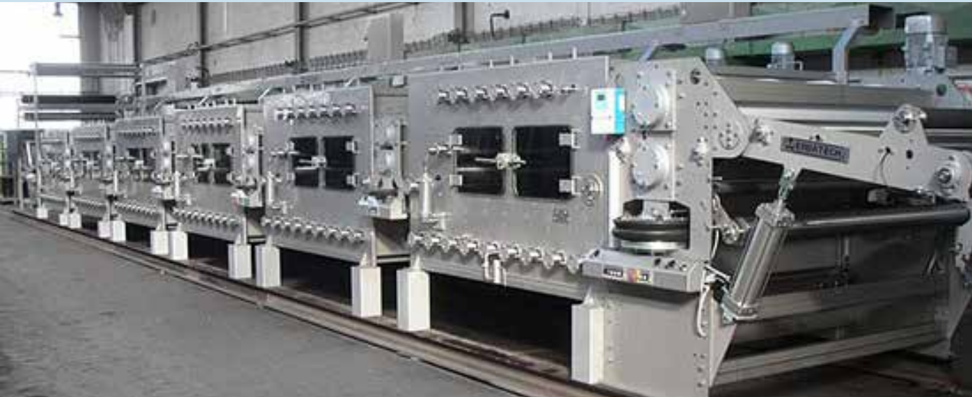
Figure-19: Wash boxes of continuous pre-treatment machine for woven fabric in counter-current washing mode
