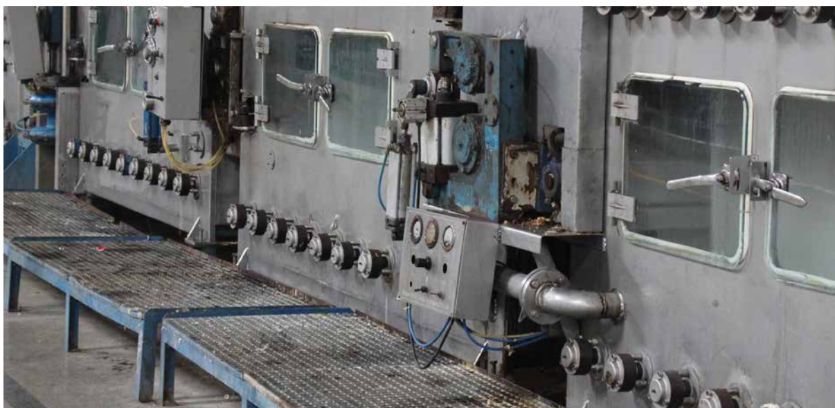
Figure-8: Three counter-currently operated washing boxes for desizing as part of a continuous pre-treatment machine (line)
