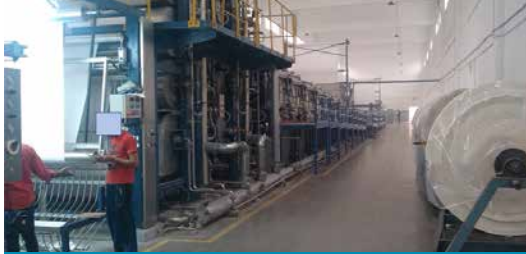
Figure-11: Example for mercerization machine for cotton woven fabric
