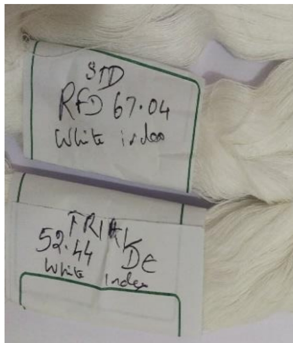
Pretreatment - Standard (top) vs TRAIL Samples (Bottom)
