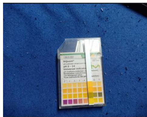
pH paper use for measuring pH before dyeing of polyester part.
